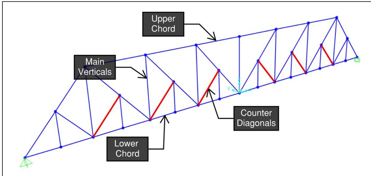
**Figure 10:** Truss Span modeled in SAP2000
